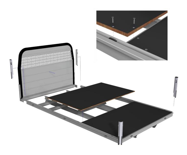
Mount the front wall and rivet the preassembled corner joints to the side edge profiles.
